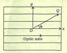
A calcite plate is cut parallel to the optic axis. Plane polarized monochromatic light is incident normally on the plate. Find an expression for resultant vibration after emerging out of the plate.
