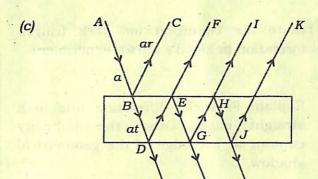
In the above diagram a transparent film of thickness t is illuminated by a monochromatic radiation. A series of reflected and transmitted rays are formed due to multiple reflection and transmission. Find an expression for resultant intensity when reflected rays are superposed. [Take r as reflection coefficient in first medium; r' is the reflection coefficient in film; t is the transmission coefficient in film and t' is the transmission coefficient in first medium.]
