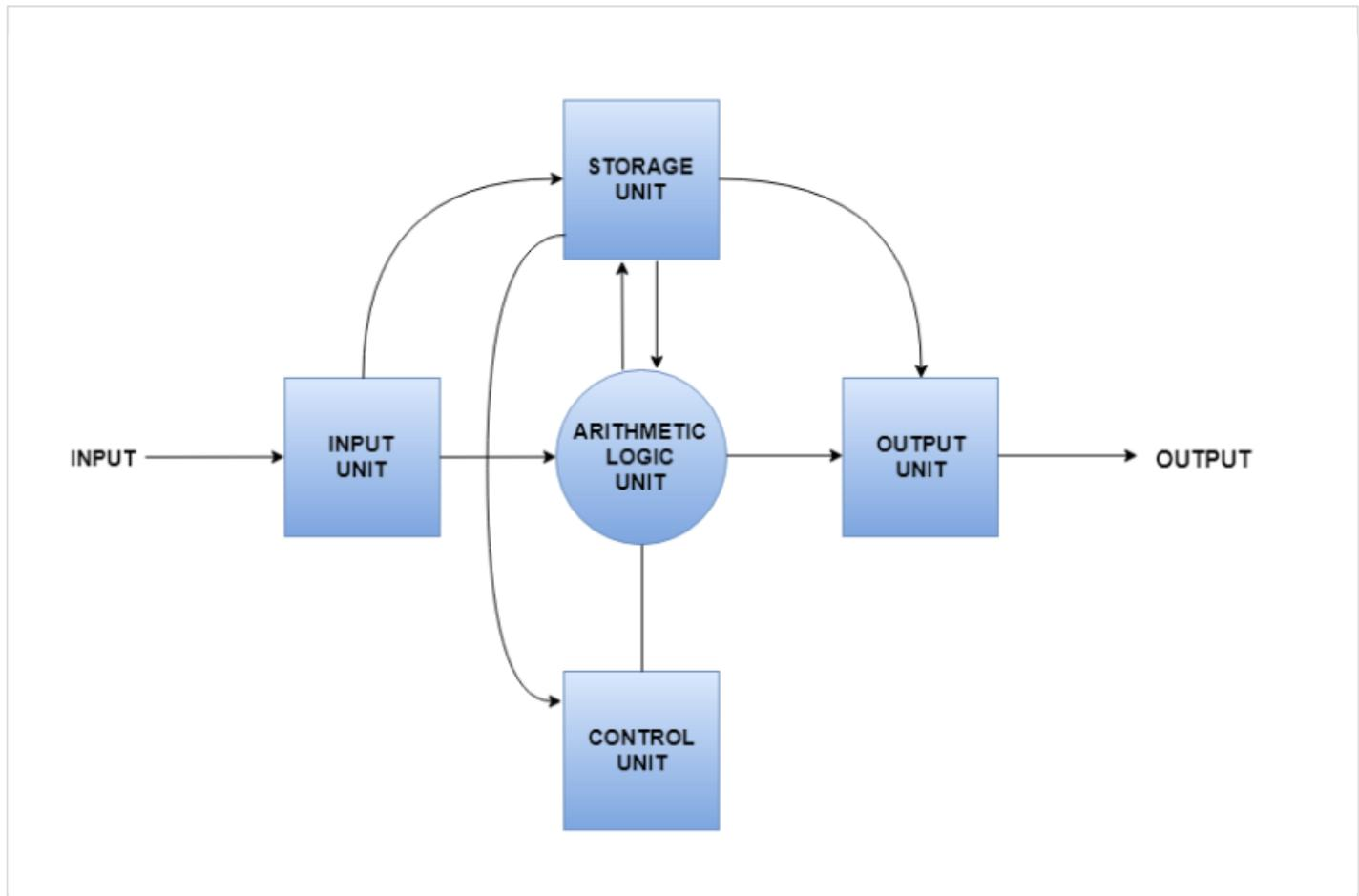
The input data travels from input unit to ALU. Similarly, the computed data travels from ALU to output unit. The data constantly moves from storage unit to ALU and back again. This is because stored data is computed on before being stored again. The control unit controls all the other units as well as their data.
