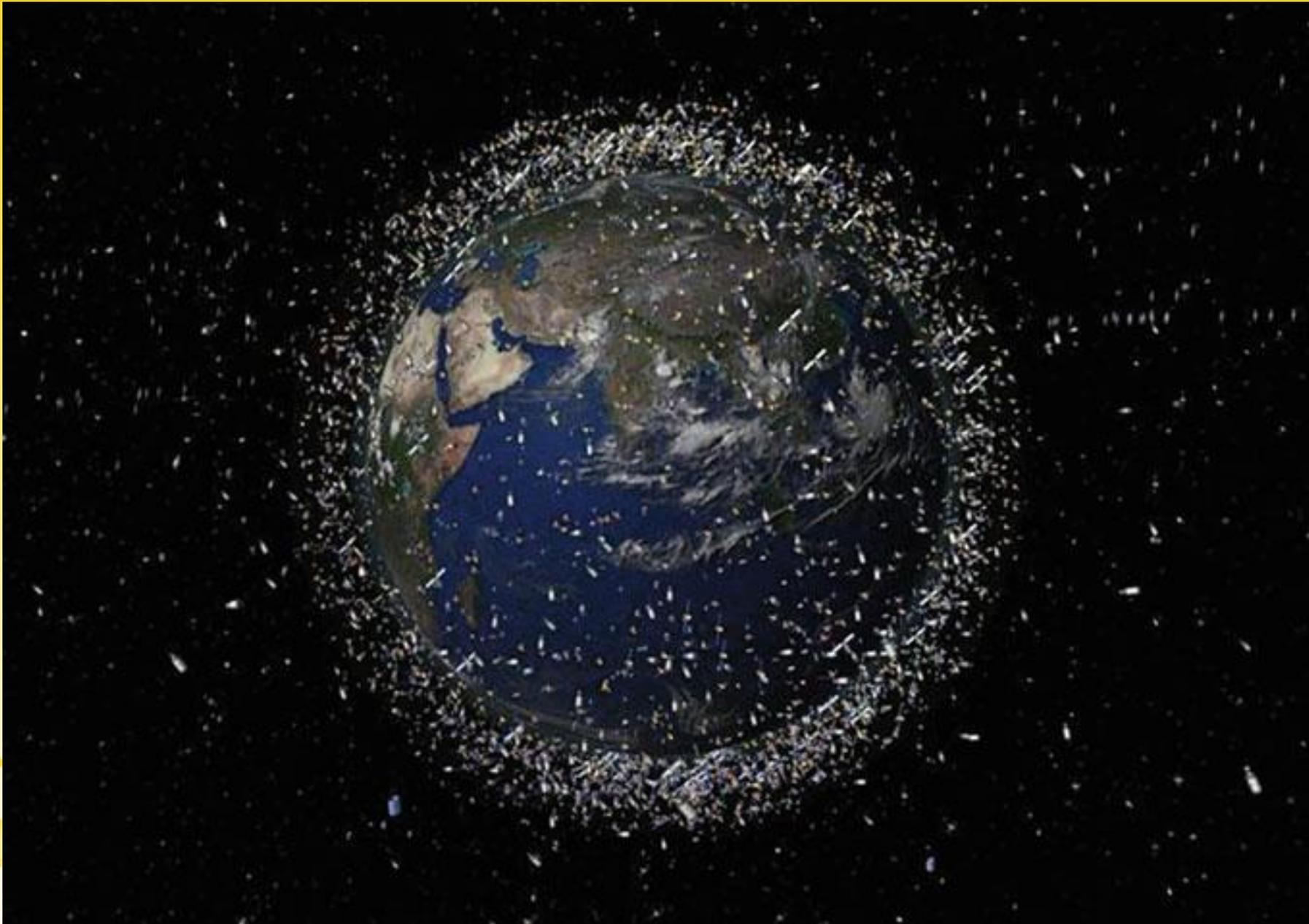
Debris objects in low-Earth orbit. These debris are largely comprised of inactive satellites and other hardware, as well as fragments of spacecraft that have broken up over time. (Objects are not to scale.) Image courtesy of the European Space Agency
