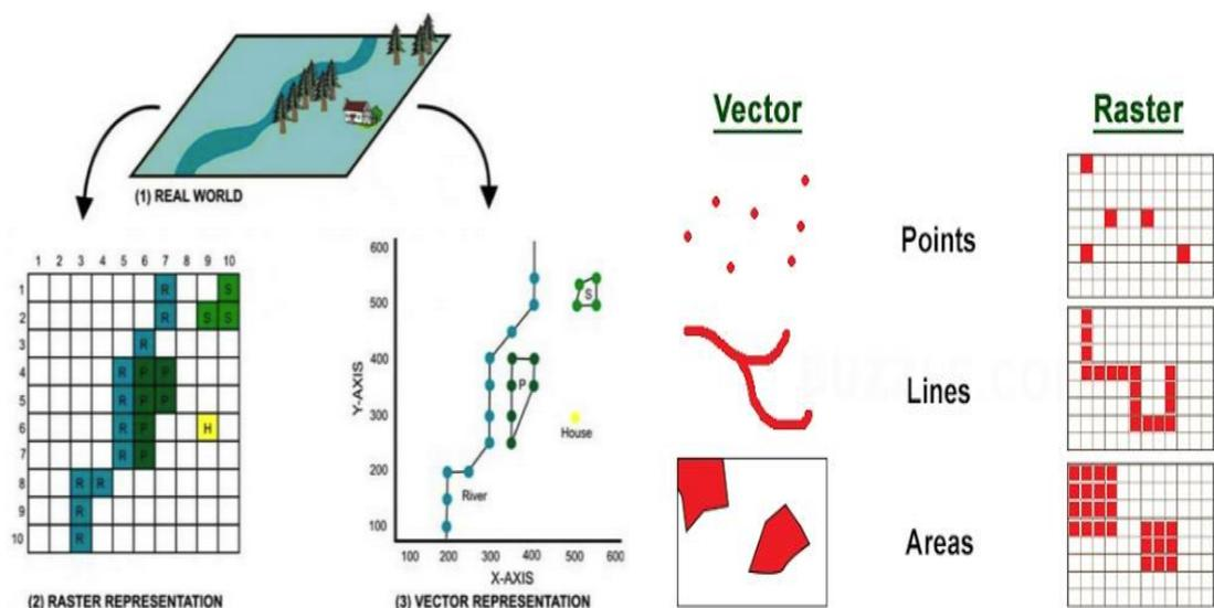
**VECTOR DATA STRUCTURE:** The basis of the vector model is the assumption that the real world can be divided into clearly defined elements where each element consists of an identifiable object with its own geometry of points, lines, or areas (polygons). In principle, every point on a map and every point in the terrain it represents is uniquely located using two or three numbers in a coordinate system, such as in the northing, easting, and elevation in Cartesian coordinate system.
