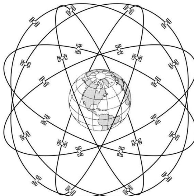
Fig: The GPS constellation 'birdcage' showing the 24 orbiting satellites
