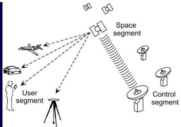
**The space segment:** The space segment consists of the constellation of spacecraft, and the signals that are broadcast by them, which allow users to determine position, velocity and time. The basic functions of the satellites are to:
